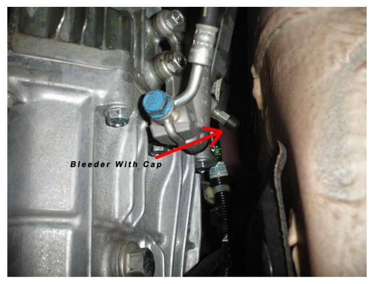
Grab your clear hose and put one end over the bleeder. Grab your 5/16 wrench and loosen the bleeder. The fluid will begin to come out right away. In my case the clear hose I was using was a little bigger then the bleeder, so it wouldn't hold firmly onto it. However, honda was kind enough to include a nice holding point for your clear hose that will keep it in place over the bleeder. At least this is the way I do it, and easiest way in my opinion. (Pic Below)
