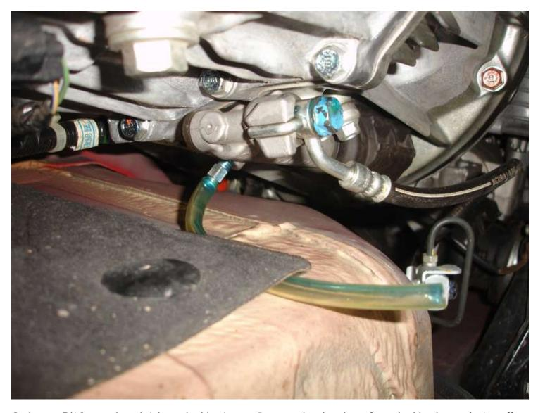
Grab your 5/16 wrench and tighten the bleeder up. Remove the clear hose from the bleeder, and wipe off any excess fluid. Pop the rubber cap back onto the bleeder. Your almost done. Lower the car to the ground. Grab your new fluid and fill the reservoir to Max. (Pic Below)
