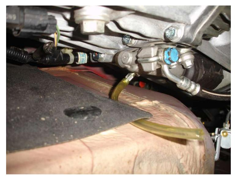
While it's bleeding the old fluid out you want to make sure to check the reservoir. The clutch bleeds very quickly, especially if there is air in the system, and you'll want to add more new fluid as it does. Keep the fluid level at Max. Within a minute or two you will start to see the new fluid bleeding out. Mine was a nice rich blue. (Pic Below)
