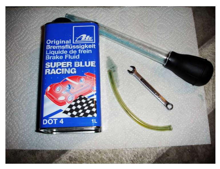
Alright let's get started. The first thing you want to do is remove the cap from the clutch cylinder reservoir(put the cap aside for now as the reservoir will be left open for the duration of the bleed) and begin sucking out the old fluid using the turkey baster. (Pic Below)
